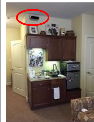
Figure 1. The Foresite Healthcare integrated depth sensor embedded system mounted in a kitchen area of an apartment (circled).
