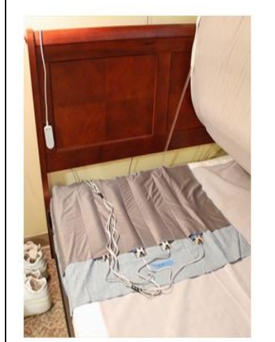
Figure 2. The hydraulic bed sensor positioned under the mattress
